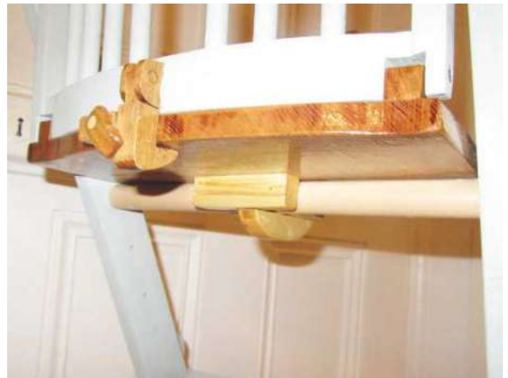
▲ Pic. 5 The main weight of the seat – and baby – is held by a thick beech rod. Two blocks beneath the seat drop over the rod, and secure it with a sturdy turnbuckle
